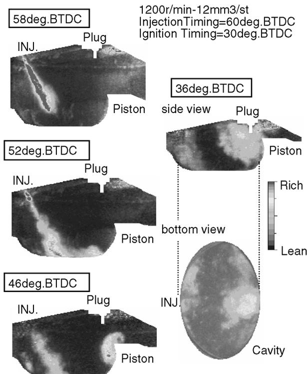
Figure 4. Fuel spray motion and mixture distribution (LIF measurements)
