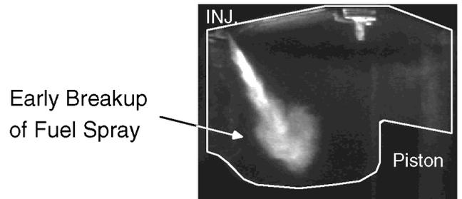
Figure 6. In-cylinder spray photograph of early breakup injector
