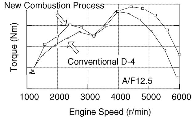
Figure 19. Torque improvements at WOT conditions
