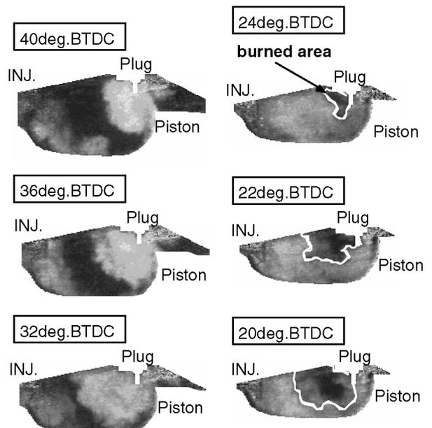
Figure 7. Mixture motion and flame propagation images of early breakup injector (LIF measurements)
