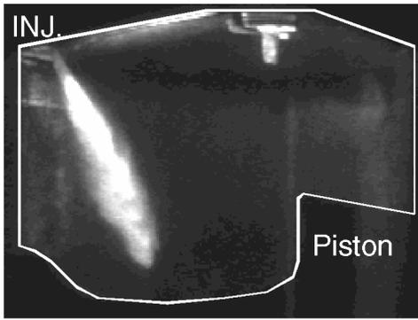
Figure 10. In-cylinder spray photograph of late breakup injector
