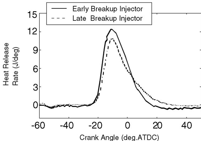
Figure 12. Effects of injectors on heat release rate
