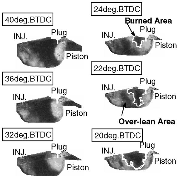
Figure 11. Mixture motion and flame propagation images of late breakup injector (LIF measurements)
