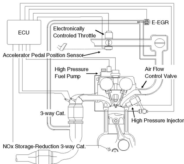
Figure 21. Schematic diagram of DI system
