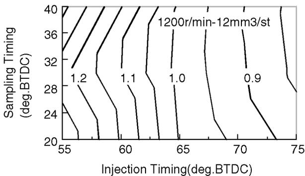
Figure 8. Equivalence ratio nearby spark plug (Fast response gas sampling)
