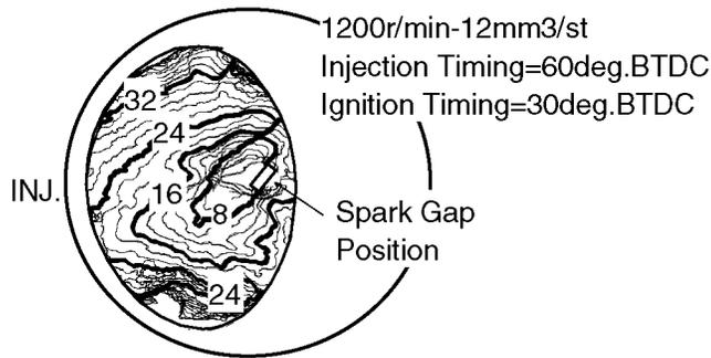
Figure 13. Flame propagation contour of cavity A
