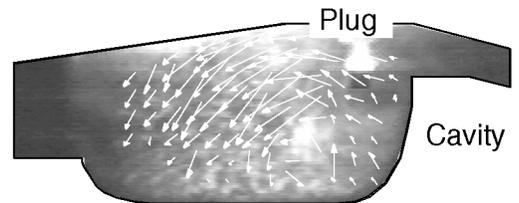
Figure 5. In-cylinder flow pattern
