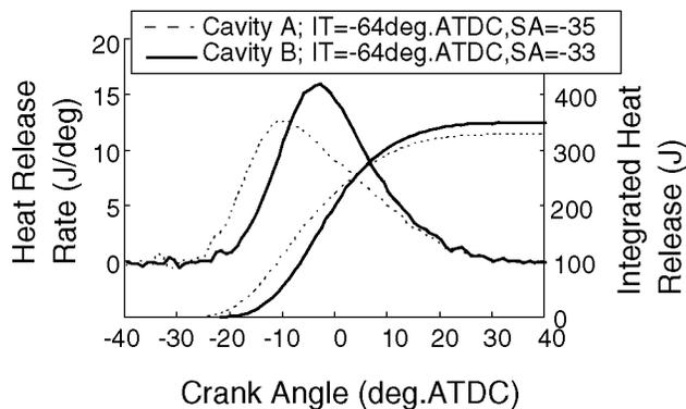
Figure 15. Effects of cavity shapes on heat release
