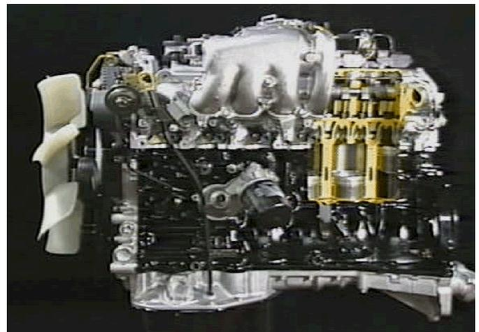
Figure 20. A New DI gasoline engine
