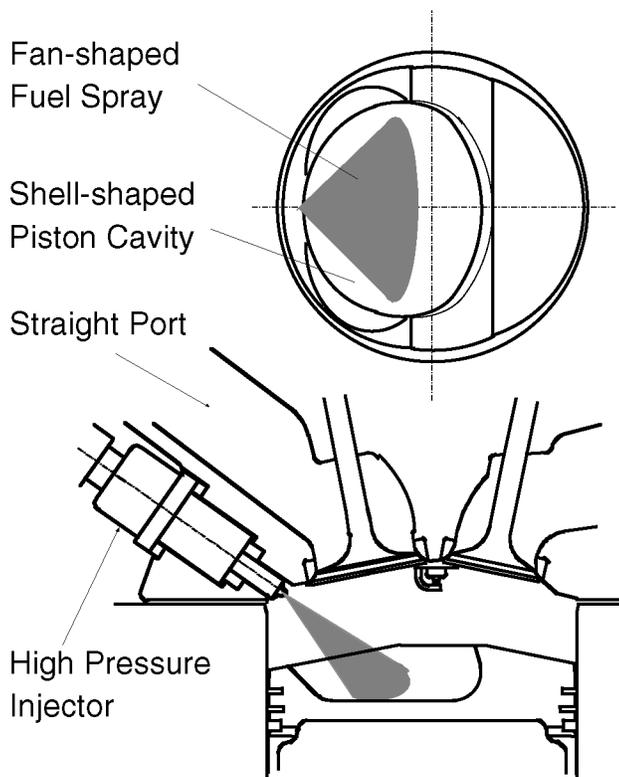
Figure 1. Fuel spray and piston cavity configuration
