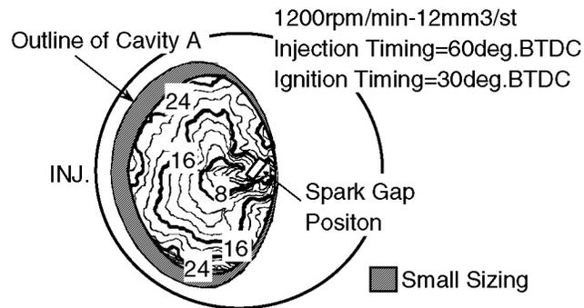
Figure 14. Flame propagation contour of cavity B
