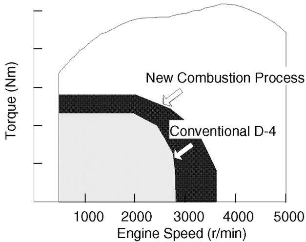
Figure 17. Comparison of stratified combustion area
