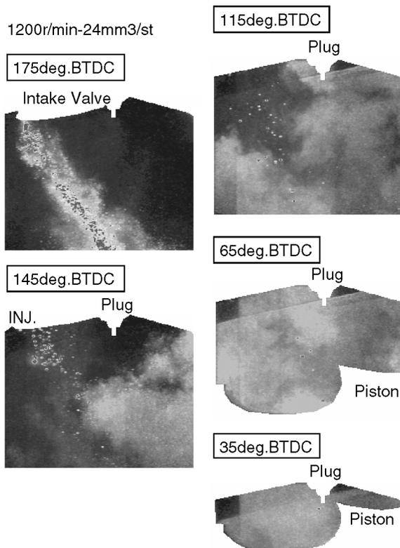
Figure 18. In-cylinder mixture distribution a intake stroke injector (LIF measurements)
