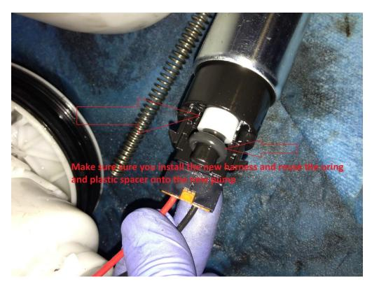
Step 7: Cut the stock connector and crimp it to the new harness. Red to blue. Black to black
