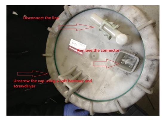
Step 3: Pull up the fuel pump assembly and remove the fuel sender line.
