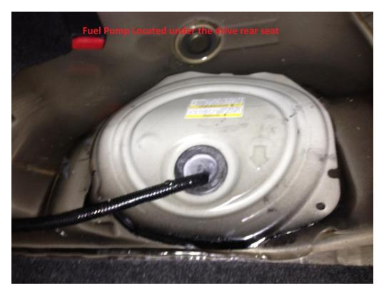
Step 2: Disconnect the fuel line and remove the fuel pump connector. Then unscrew the lid using a flat had screw driver and soft hammer.
