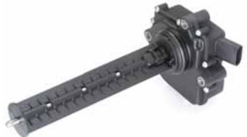
The intake manifold tuning valve separates the intake plenum into halves, with each bank of the engine breathing through its own half at lower revs for improved torque, but opening to provide access to the entire intake manifold volume at higher rpm for maximum top-end power.
