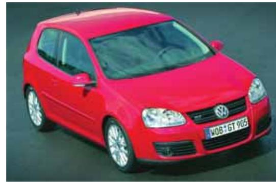
Beneath the hood of the VW Golf GT is a 1.4-L Twincharger engine producing 125 kW (168 hp) and 240N·m (177 lb·ft).
