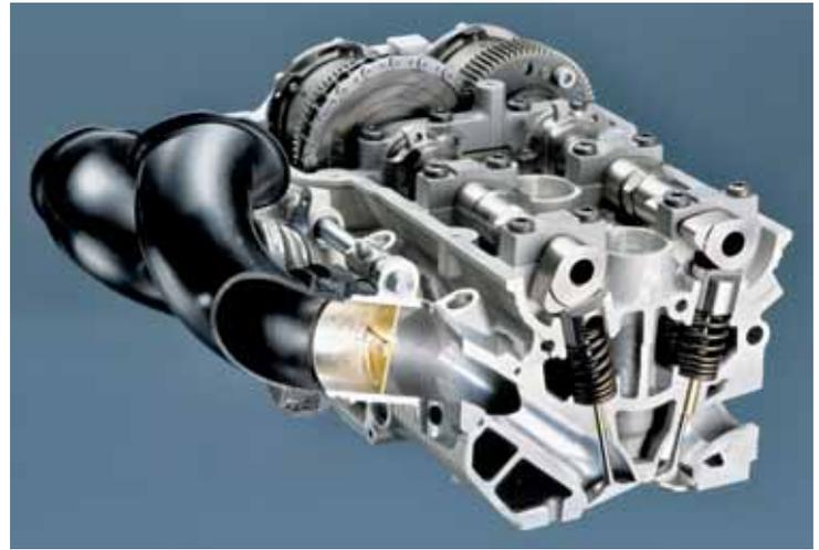
Special attention was paid to reducing mass in the M5's valvetrain, resulting in a total mass reduction of 17.5% compared with the preceding V8 engine. The hydraulic tappets, for example, acting on each cylinder's four valves, were trimmed to just 28 mm (1.10 in) across, with a mass of 31 g (1.1 oz).
