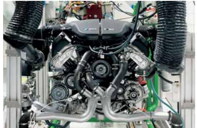
To ensure continuous quality, each of the hand-assembled M5 engines runs for 20 min on a dynamometer to confirm its correct operation, and some engines are tested randomly for two hours.
