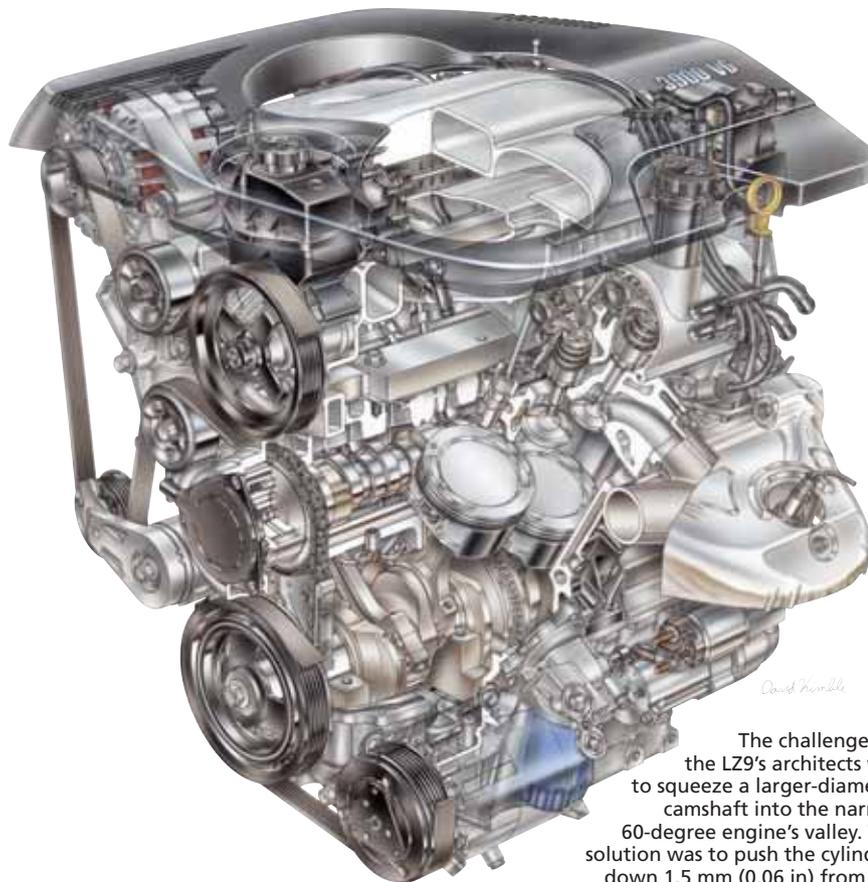
The challenge for the LZ9's architects was to squeeze a larger-diameter camshaft into the narrow 60-degree engine's valley. The solution was to push the cylinders down 1.5 mm (0.06 in) from the top of the block, widening the area where the cam resides.
