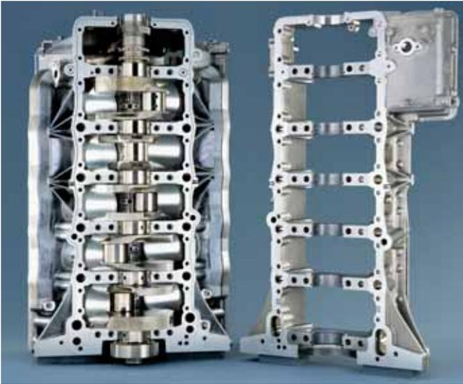
The cylinder block is low-pressure gravity die-cast of hypereutectic aluminum-silicon alloy containing 17% silicon. This material permits the creation of cylinder liners by precipitating hard silicon crystals, eliminating the need for pressed-in liners.
