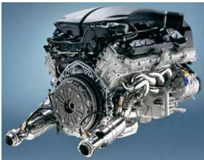
Like the predecessor M5 V8, the new V10 displaces five liters of capacity and has a mass of about 240 kg (529 lb), but the new engine's extra pair of cylinders and additional 1250 rpm contribute to a 107 hp (78 kW) hike in output.
