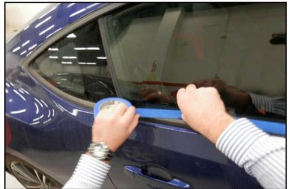
Figure 3. Example of Tape Applied to Front of Outer Door Weatherstrip
