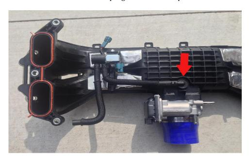
The red highlighted area is the vacuum line to the break booster. This also can be used as another vacuum source
