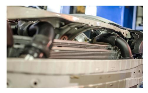
B. Cold side consists of 2.25" coupler, 2.25" Aluminum 90\*, 2.25"-2.75" coupler, 2.75" Aluminum MAF pipe with BOV flange, and 2.75"-3" Coupler in that order
