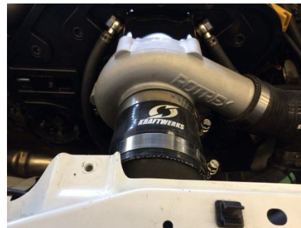
Figure 53: 3" coupler connecting supercharger inlet to intake tube
