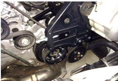
Figure 23: Belt routed around the lower pulley
