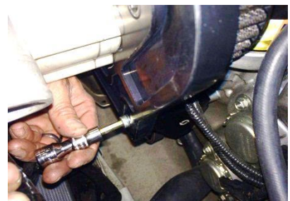
Figure 19: Torque (2) M6 bolts to 20 ft-lbs that goes into lower support bracket
