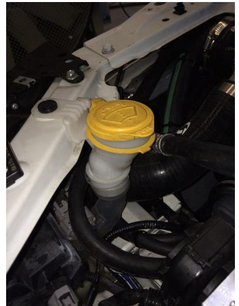
Figure 41: Factory fill neck installed in new reservoir
