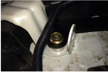
Figure 30: Reservoir support bracket bolted to car
