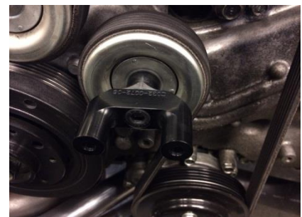
Figure 9: “Y” support bracket installed (Do not tighten bolt yet)
