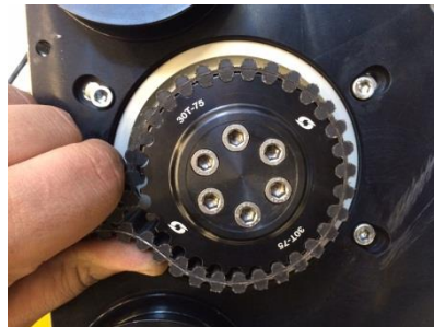
Figure 15: How to hold pulley from spinning using the belt
