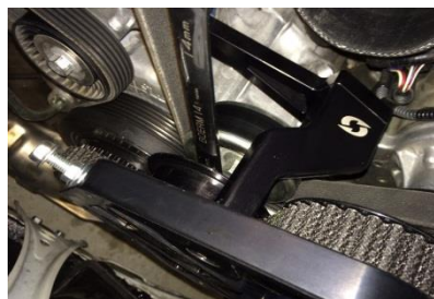
Figure 26: Tighten the Idler pulley
