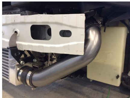
Figure 47: Hot side charge tube installed
