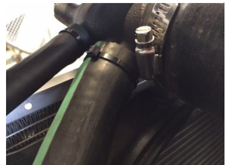
Figure 60: Crank case breather and bypass valve recirculation hose connected to intake
