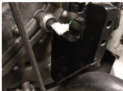
Figure 11: Lower support bracket installed (Do not tighten bolts yet)
