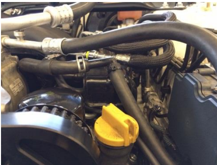
Figure 59: Crank case breather extended
