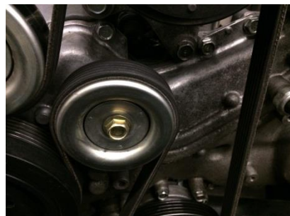
Figure 8: Remove the factory bolt from the idler pulley
