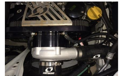
Figure 38: Oil line routing and fittings in supercharger
