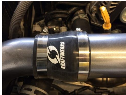
Figure 50: 2.5" to 3" reducer between second and third charge tube
