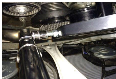
Figure 24: Adjust Tensioner bolt until you have 21MM between plate and bolt
