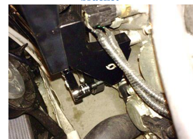
Figure 21: Torque the (2) M6 bolts that hold the Lower support bracket to block to 9 ft-lbs
