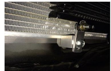
Figure 35: Oil cooler installed on A/C condenser
