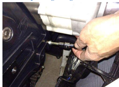
Figure 18: Torque (2) M6 bolts to 20 ft-lbs that goes into the “Y” support bracket
