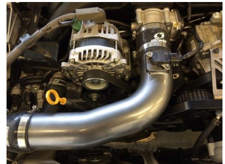
Figure 51: Third cold side charge tube installed
