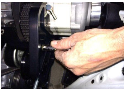
Figure 17: Torque M10 bolt to 38 ft-lbs that goes into upper support bracket
