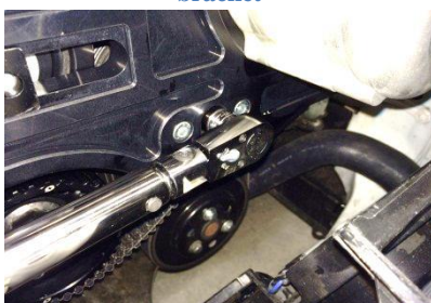
Figure 20: Torque the M10 bolt that holds the “Y” bracket to block to 38 ft-lbs
