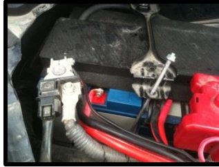
Loosen/ unhook tie bolt and slide back cover to expose 24V positive lug.
