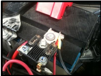
Re-install tie bolt, tighten. Attach the yellow eyelet to positive clamp bolt. Connect Neg clamp.
