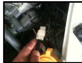
From the battery: run the long cable along the strut brace (zip tie) toward the AUX. Connect White.
