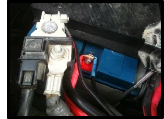
*Disconnect neg factory clamp (not shown) Remove nut/ attach blue eyelet to 24V POS.
