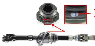
The new part has 6mm diameter white marking on the dust cover.
