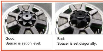
4-4 Set COLUMN ASSEMBLY-STEERING as shown in the below photo.
