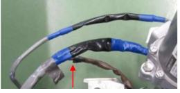
Bad: Vinyl tape is removed and harnesses are separated.
