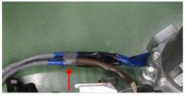
Good: Vinyl tape holds all wiring harnesses together.
