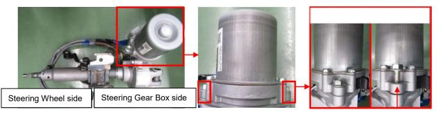
Loosen two tightening bolts.
