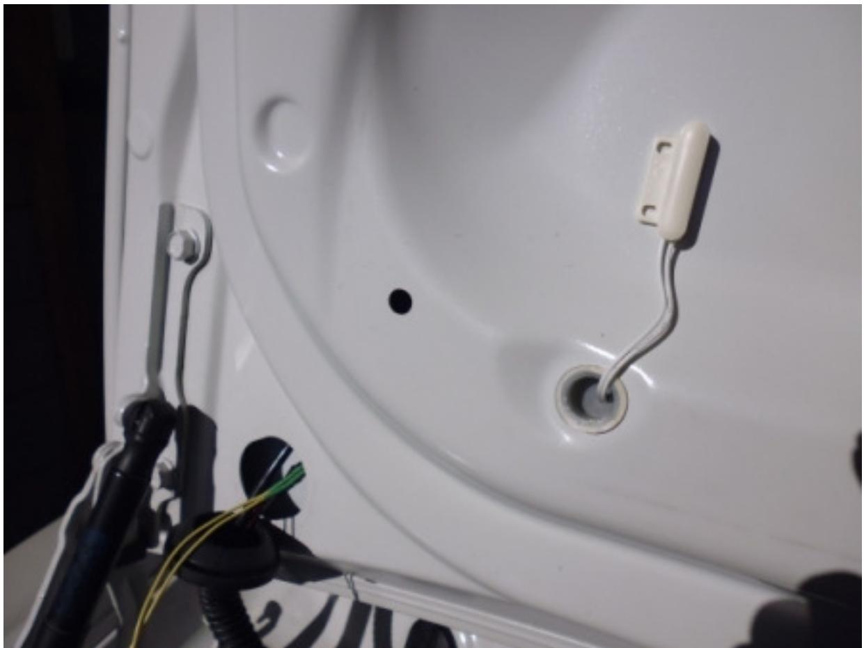
Attach the switch to the boot lid in the position shown with the supplied double sided adhesive pad supplied with the switch. I lengthened the wires by about a metre so it will reach the light. If you happen to have a plastic bung or something similar to plug the hole where the wires go through, then use it. However it is not essential providing there are no sharp edges. Pull out the OEM rubber boot so you can thread the new wires into it, leading to the light.
