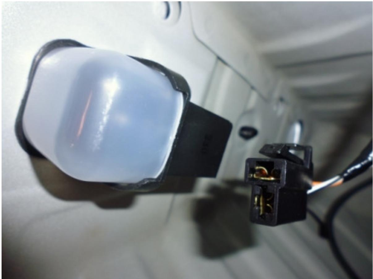
Unplug the connector from the light. **\*\*Also unplug the connector from the boot release mechanism to isolate the light connector from ground.** Note that the Orange/White wire will still have +12V on it. If in any doubt while working "LIVE" on this, then disconnect the battery!
