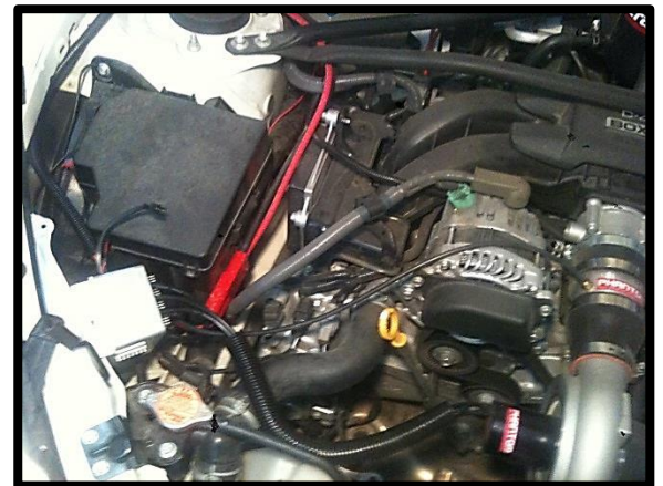
STEP 18: Run large cable from 24V battery under strut bar and toward the controller. Run +/- eyelets from controller to battery area.
