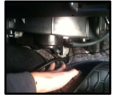
STEP 21: Route 6 pin connector through sound tube passage into engine bay, sound tube must be removed. Pull WIRES behind the connector to controller.
