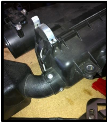
STEP 2: Disconnect OEM battery, remove battery. STEP 3: Remove intake from airbox to throttle body. STEP 4: Remove air box by removing 3 bolts. STEP 5: Drill rivets out, 3/16", remove resonator (picture).
