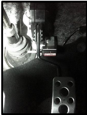
STEP 19: Bolt on PWS as shown. Use OFT throttle % readout to adjust 60-70% 1 st click... 2 nd click will occur 90-100%. Push or pull to slightly yield finger till desired % is achieved.
