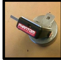
Part/WOT switch (PWS). Partial is trimmable (screw, 0-50% boost)
