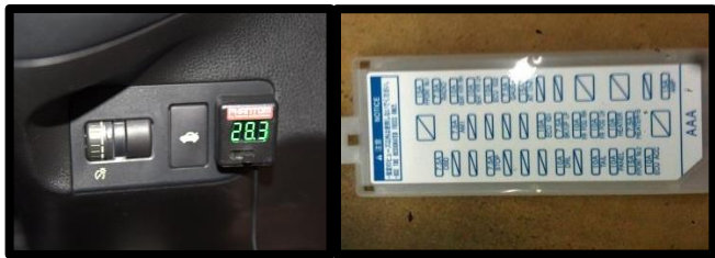
STEP 22: Position LED display as shown Run red ATM fuse to fuse box located under steering colum, between DRL and TAIL. Connect RED jack to PWS...BLACK jack to Voltmeter. ZIP TIE cables.
