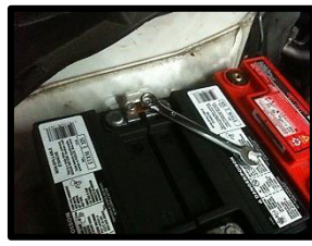
12: bolt on copper series connector (Always remove Cu when working on +/- main)
