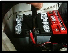
11: Drop in battery tray. Arrange three batteries as shown. Bolt on heavy gauge cable (+,-)
