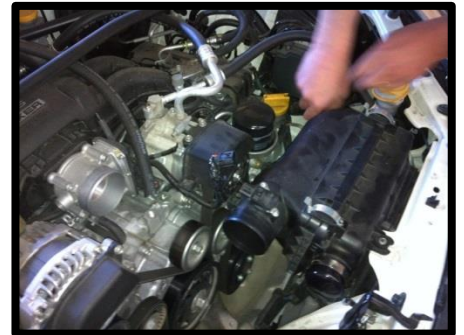
STEP 7: bolt airbox using 2 bolts.
