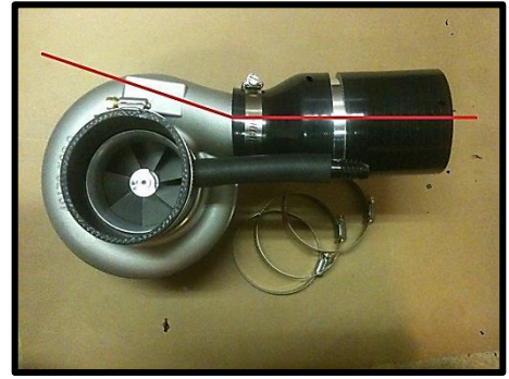
STEP 1: Assemble silicone, position as shown. attach hose clamps.
