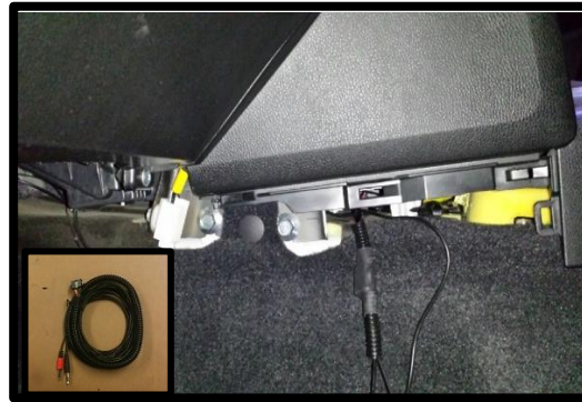
STEP 20: Remove lower center console panels. Run the 6 pin connector through to the passenger footwell. Do not pull on 6pin connector, pull on wires, * harness can be feed from engine bay as well...jacks 1 st .
