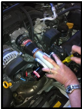
STEP 8: Attach compressor unit. Hold unit in place while tightening.
