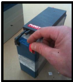
Place series block as shown, press connectors on F2 terminals. Make sure they are seated tight, tape as shown.
