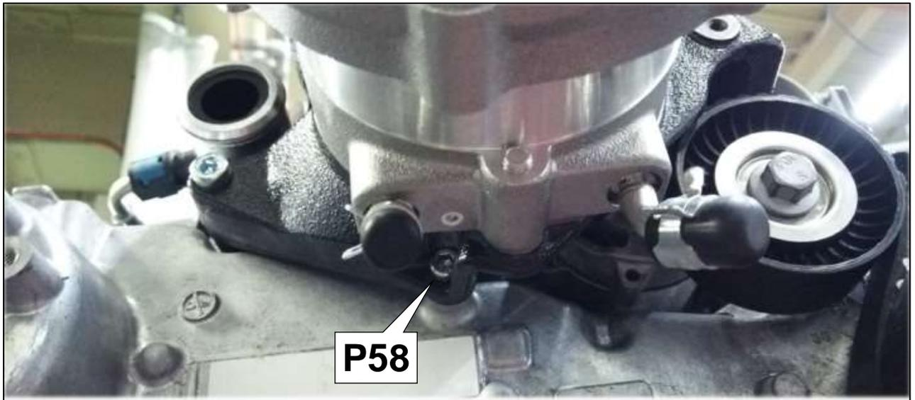
(4) Install ⑩ oil level gauge modified in 2.(27) to the Supercharger Bracket and engine using the Oil Level Gauge Clamp.
