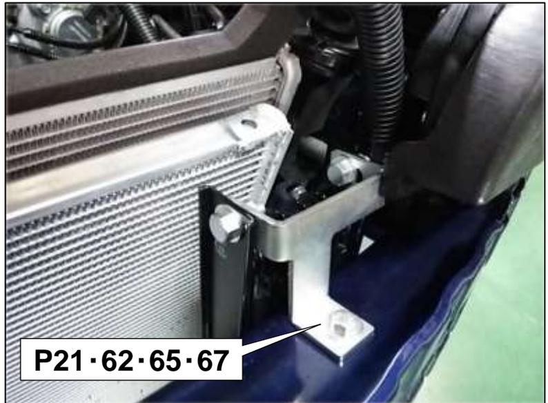
(16) Install the Traction Fluid Tank to the ① radiator support modified in 2.(14) using the following provided parts.
