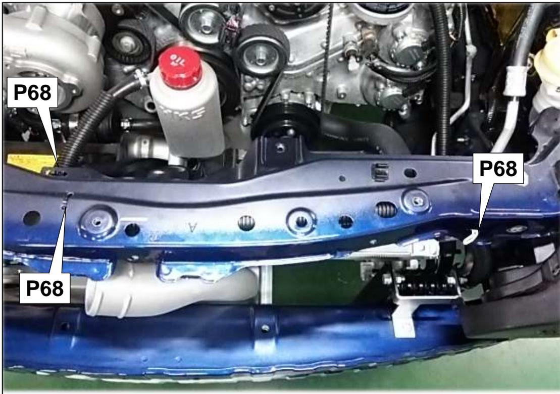
(19) Secure the Traction Fluid Hose 8mm ② to the Radiator Support in the position shown in the diagram above using the provided Tie Wraps (M). Pass the Tie Wraps through the holes made in 2.(14) and ones originally existed.
