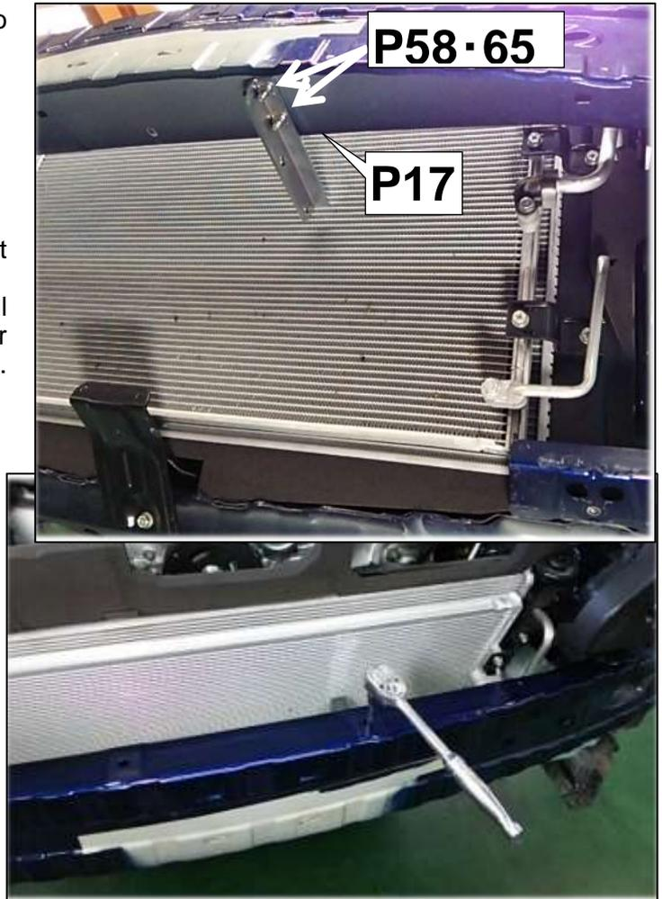
(5) Shave 2mm of the pipe clamp on the A/C condenser of the passenger's side as shown below.
