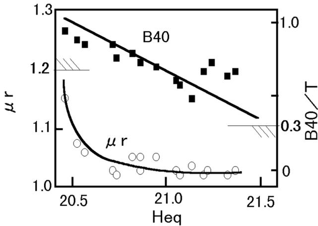
Figure 7. Variation of Magnetic Properties as a Function of Hirayama's Ni equivalent: Heq
