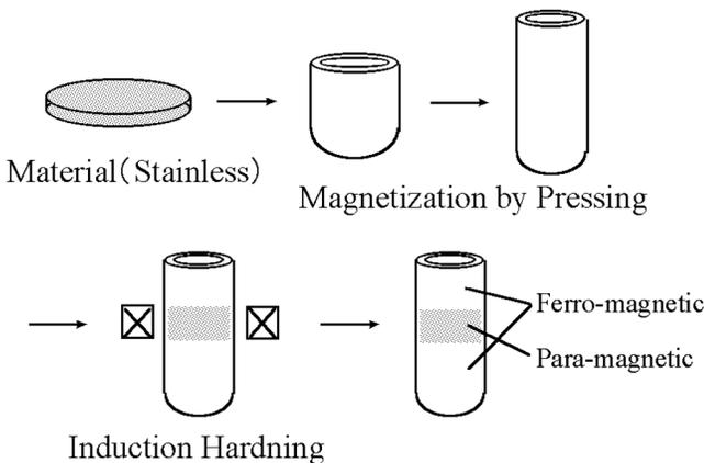
Figure 8. Composite Magnetic Material
