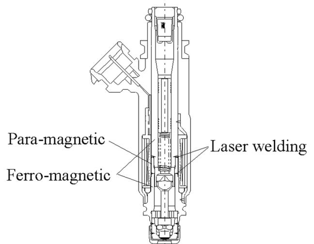
Figure 6. Injector for Port-Injected Engine
