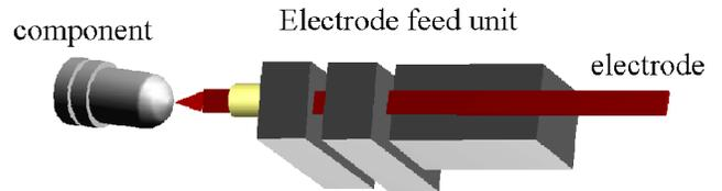
Figure 13. Fine Electric Discharge Processing
