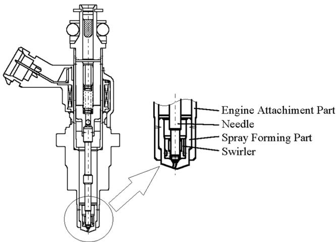
Figure 10. Construction of Swirl Injector
