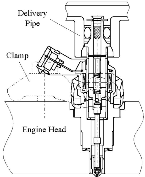
Figure 3. Installation of the Injector
