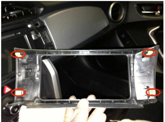
Pull off the head unit trim panel. If you have a plastic wire/panel tool, this might help. I was able to pull this out simply with friction from the pair of vinyl gloves that I was wearing. Do not use a metal pry tool (certainly not a screw driver) so as to not scratch the trim panel.
