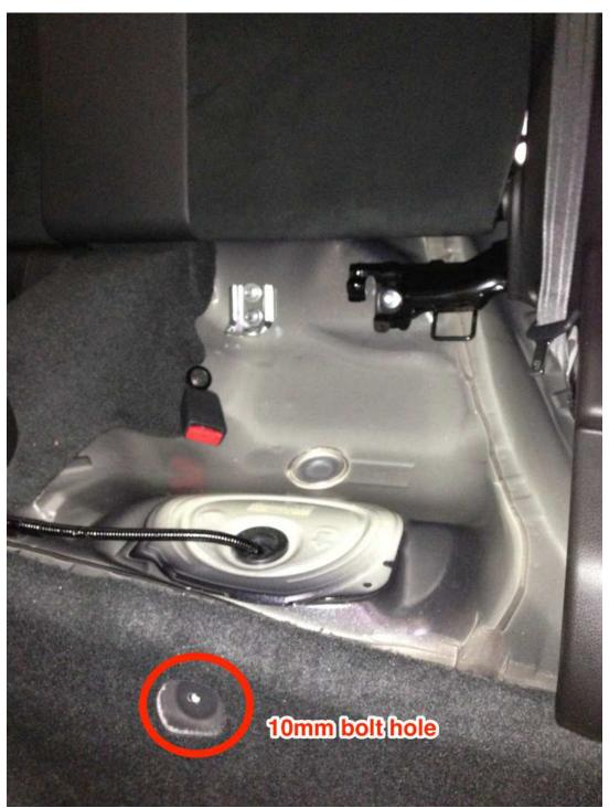
Using a 10mm socket, remove the bolt holding the driver's side rear seat bottom in place. Firmly push on the back side of the seat bottom and slide the seat off.
