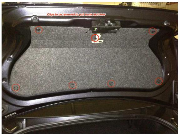
In my car, there's a carpet covering the roof of the trunk. You will need to remove this by popping the seven clips holding it on. Gentle pry the center of the clip out using the tip of a flat blade screw driver. Once you loosen the clip, it may not be easy to pull the clip out, in this case, gently lift the carpet away from the trunk (just make sure the clip doesn't go flying off). Set the carpet aside.
