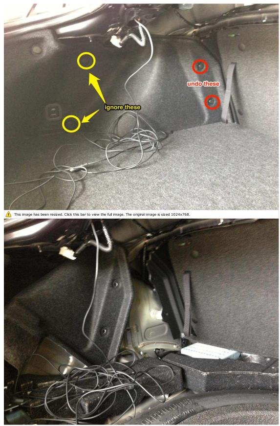
Remove the two clips in the trunk holding the driver's side trunk liner to the body. Fold the trunk liner back but do not remove the trunk liner (there's still two clips holding it on
