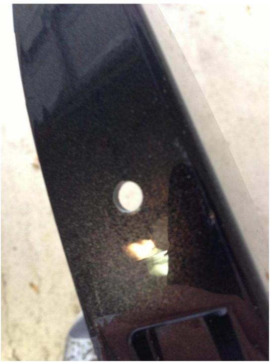
Now drill the hole, for my camera, I needed a 1/4" drill bit. Be careful not to over-drill and damage any other part of the trim. Clean up the edges of the drilled hole with sand paper to avoid sharp edges (this is optional, but again, I'm going for completeness).
