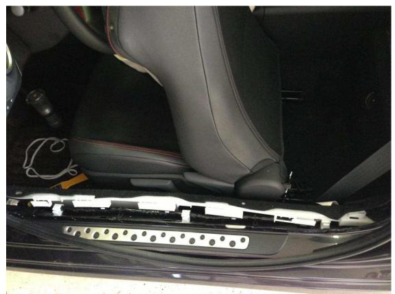
Now remove the door threshold trim. Pull gently along the edges to loosen the clips holding it in. You may find that using a panel tool or something will help you pry it loose. I used a plastic putty knife. Either way, don't force it.
