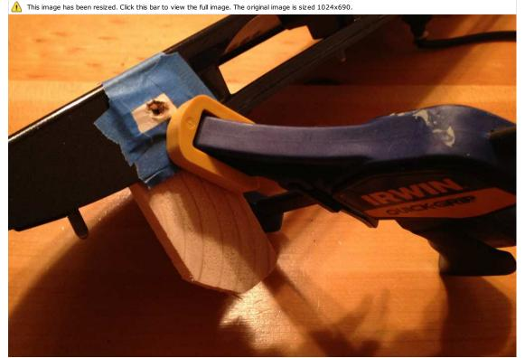
This is a woodworking trick. Clamp a piece of wood to the back of the trim piece to prevent splintering the back side of the hole you'll drill. It isn't strictly necessary, but you really get one shot at this so a little insurance can't hurt. Measure and make sure the hole is exactly where you want it to be (again).
