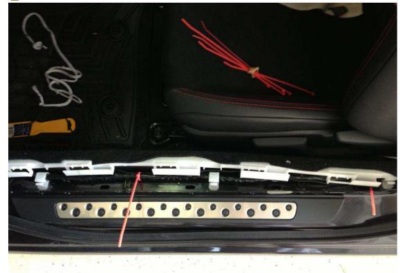
Shove a length of shoestring through the driver's side rear panel and make sure there's enough exposed on both sides. Tie the camera wire to the shoe string and use the shoe string to pull the camera wire through the gap in the panel. Work the wire along the existing factory wiring underneath capet, using zip ties to secure the camera wire.
