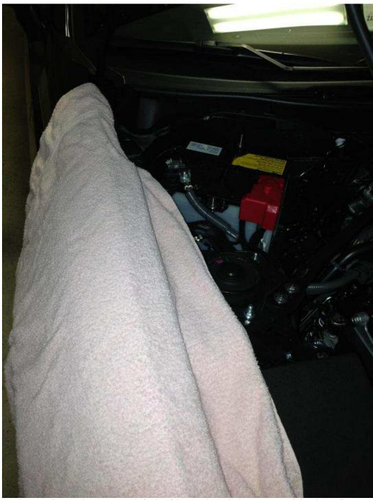
First lay a towel across the passenger-side fender of the car. Always do this to prevent a belt or button from scratching the paint.
