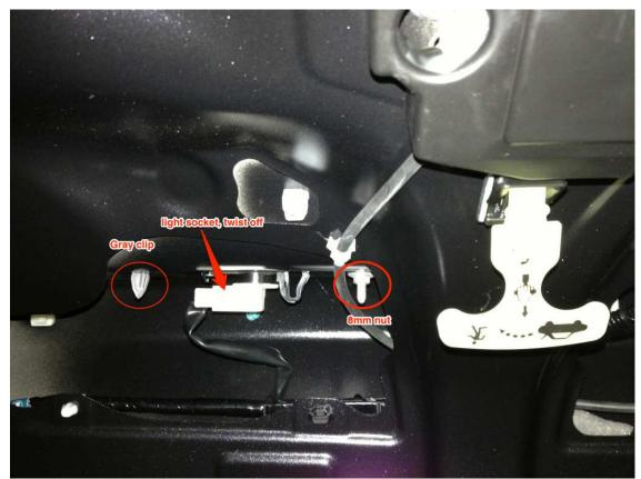
The trim piece is now attached using five 8mm nuts and a gray-colored clip. Two of these 8mm nuts are holding the trunk lock in place. Remove the two nuts holding the trunk lock (right most nuts) and gentle pull the trunk lock off and let it dangle. Now remove the three remaining 8mm nuts.
