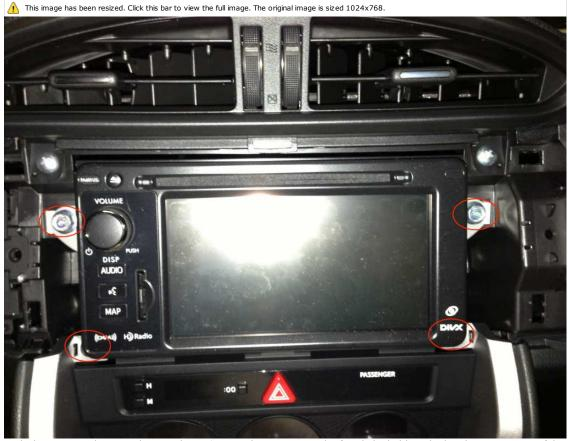
With the trim panel removed, use a deep 10mm socket to remove the four bolts holding the head unit in. Be careful not to drop any of these bolts as you will be dooooomed if you lose one (j/k, just be careful). Gently pull back the head unit and rest it on top of the towel, which is covering the shifter. You do NOT have to disconnect all of the connectors on the back of the head unit. In fact, don't because you don't want to have to remember what went where.
