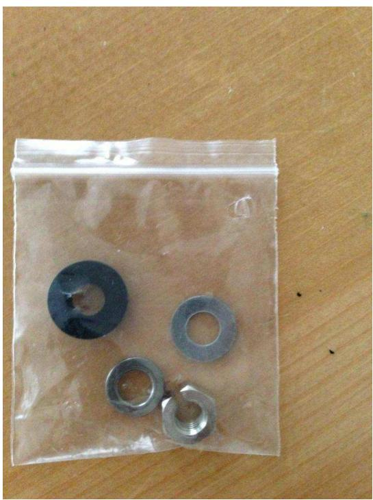
Now mount the camera through the hole. My camera came with 4 pieces of mounting hardware: a rubber gasket, a flat washer, a lock washer, and a nut. The order in which this is attached is basically this: camera, gasket, trim piece, flat washer, lock washer, nut. Position the camera how you want, once you've attached the trim piece, it will not be easy to adjust the camera so take some care here.
