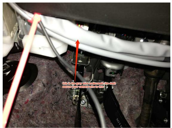
Work your way towards the front of the car. Underneath the dash, there's a thick gray wire to which you can secure the camera wire. Eventually, feed the camera wire into the head unit cavity.
