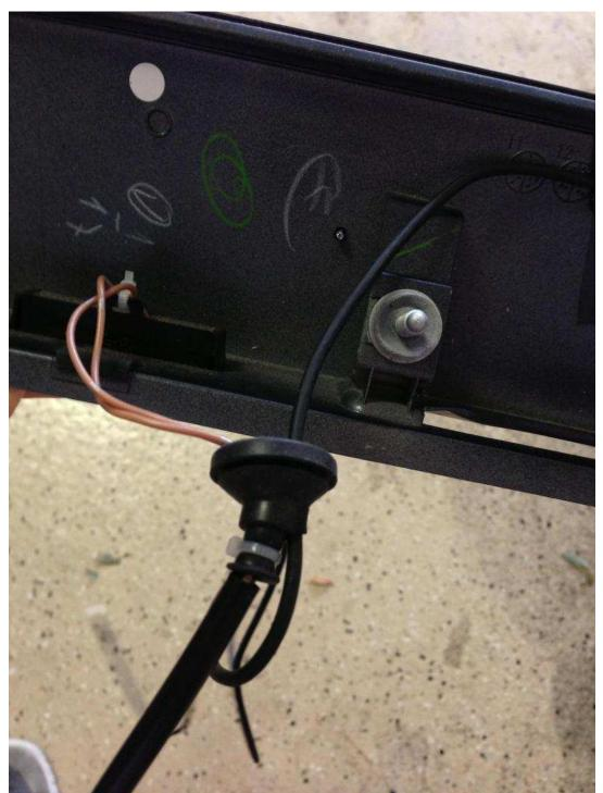
Using the straw, pass the camera wire through the grommet. Leave enough wire to provide slack should you need to pull the trim piece off the trunk later.
