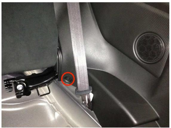
Now, remove the clip holding the driver's side rear panel (exposed by removing the rear seat bottom)
