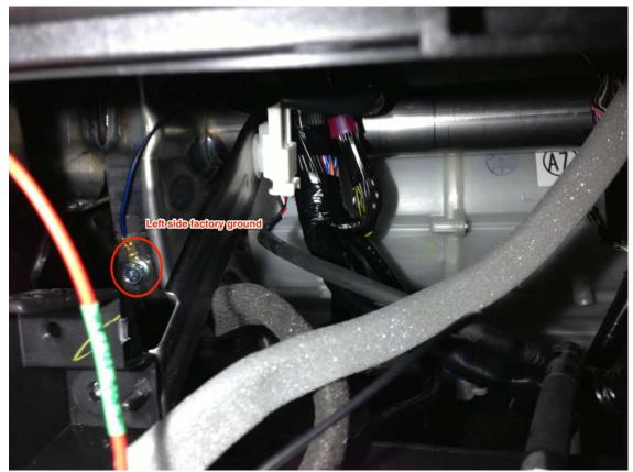
Find the factory ground location in the head unit cavity (might need a flashlight to see inside). There's one of the left and one on the right. I used the left side one because the ground wire coming off of SVXdc's harness isn't really that long and won't reach the right side ground bolt. Loosen this bolt slightly with a shallow 10mm socket. Do not pull the bolt out, definitely don't lose the bolt. You just need to loosen it enough to slide the fork terminal from the SVXdc harness onto the bolt.
