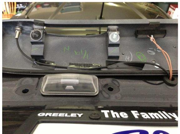
Using electrical tape, make a clean route for the wire on the inside of the trim piece to make sure it doesn't get pinched when you re-attach the trim piece. Pass the camera wire and the trunk lock button wire through the hole in the trunk and re-seat the grommet in place.
