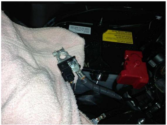
Once you've disconnected the negative terminal, cover it with the towel and put the negative terminal connector on top of the wire. The ensures that you will not have accidental power connection.
