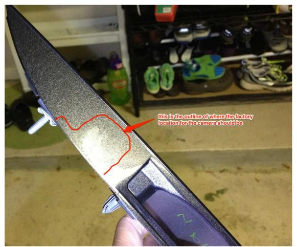
With the trim piece off, identify where you want to mount the camera. Again, there appears to be an outline on the trim piece for where a factory camera should go (the default grid line orientation of the head unit expects the camera here).
