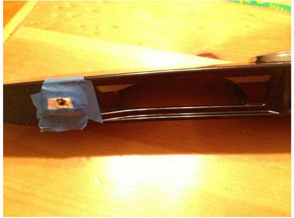
Attach your template to the trim piece using blue tape, take care to measure and make sure the camera will fit. In my installation, I placed the camera slightly towards the back of the car, in many others, I've seen the camera mounted further towards the front of your car. Ultimately, you just want to make sure that with the camera attached, it won't interfere with re-mounting the trim piece.
