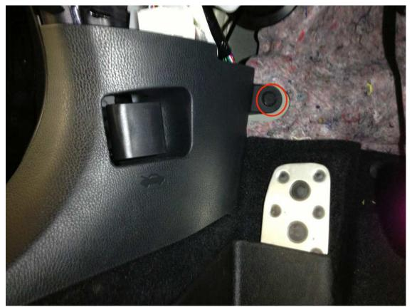
Start with the left-side kick-panel in the driver's side footwell. It's held on by one clip (similar to the clips holding the trunk roof liner). Loosen this clip and pull the panel out and back. It should come off.
