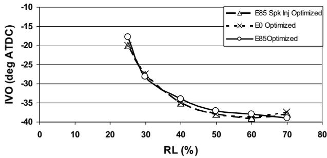
Figure 14 Intake Valve Timing Response at 3500 rpm
