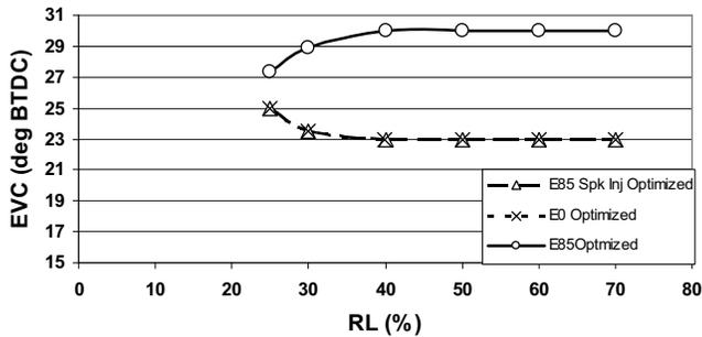
Figure 15 Exhaust Valve Timing Responses at 3500 rpm
