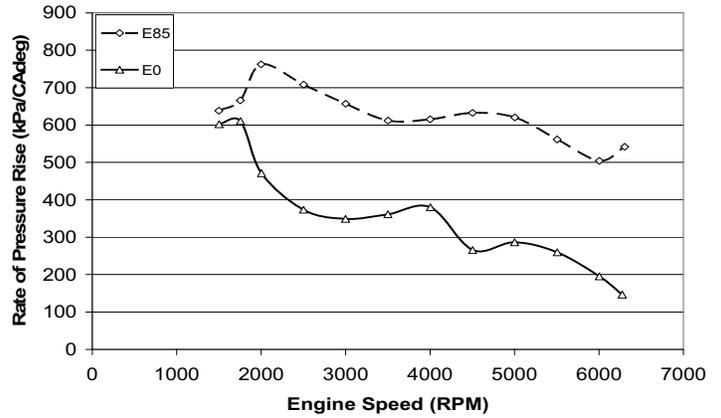
Figure 21 Maximum Rate of Pressure Rise E85 and E0
