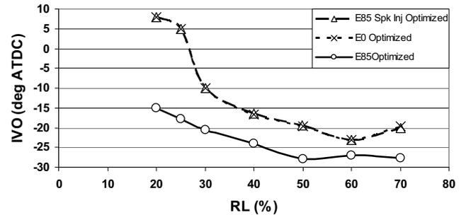
Figure 6 Intake Valve Opening Responses
