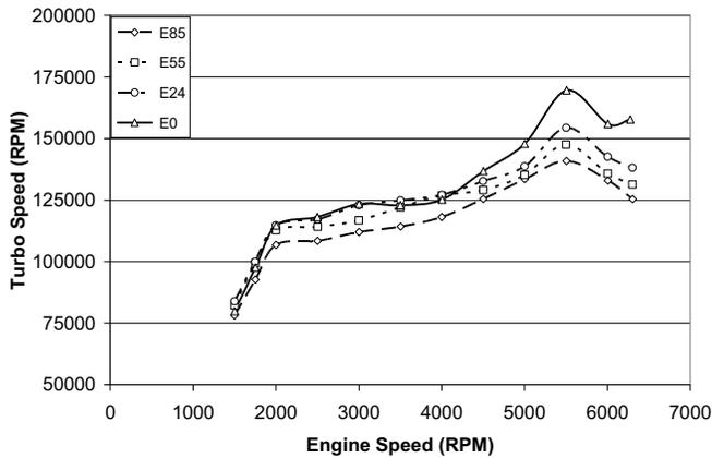
Figure 24 Turbo Speed E85, E55, E24, E0
