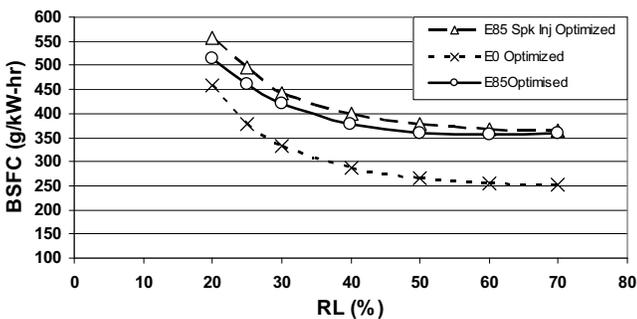
Figure 11 Brake Specific Fuel Consumption Responses
