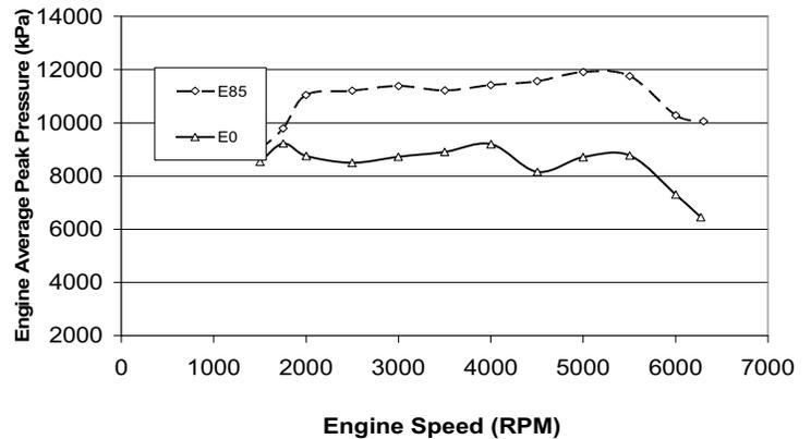
Figure 22 Maximum Peak Cylinder Pressure E85 and E0
