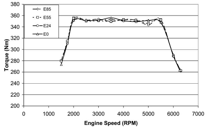
Figure 17 WOT torque curve on E0, E24, E55 and E85.
