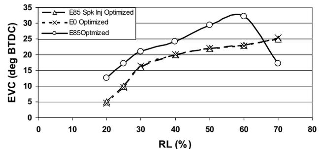
Figure 7 Exhaust Valve Closing Responses
