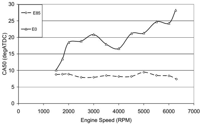
Figure 20 CA 50% Mass Fraction Burn E85 and E0.
