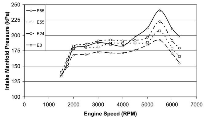
Figure 23 Manifold Pressure E85, E55, E24, E0
