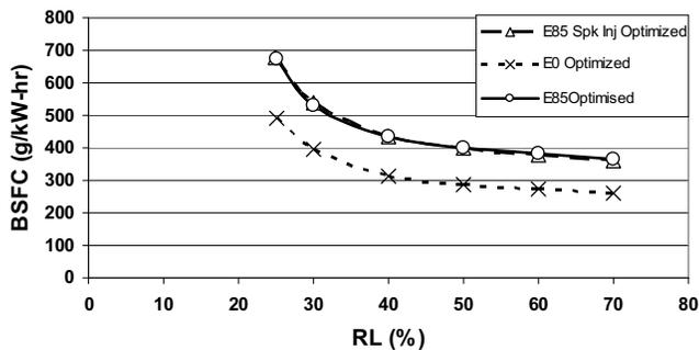
Figure 16 Brake Specific Fuel Consumption Responses at 3500rpm
