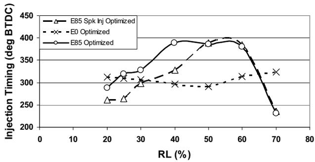
Figure 8 Injection Timing Responses
