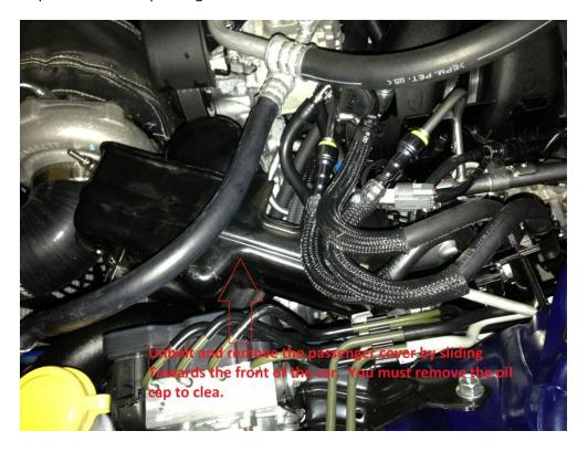
Step 3: Install will be the same for both sides once the covers are removed. Unbolt the two 8mm bolts (12mm heads) that holds the rail down. You will not be reusing these. Since the new injectors are taller, you will need to use the supplied hardware and spacers to install the new injectors.
