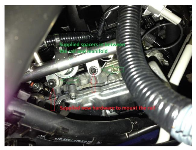
Step 5: install the injectors with the supplied hardware and use the Pnp Adapters for the wiring. Once the injectors are installed, you can put the covers back on but be careful because the connects must face a certain direction to clear the cover. The injector should spin freely between the rail and manifold.
