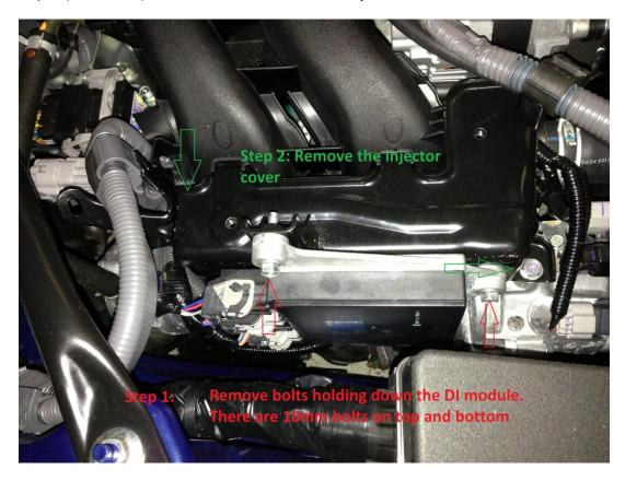
Step 2: Remove the passenger side cover
