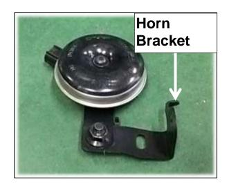
(7) Rotate the horn bracket to the position shown in the diagrams below.
