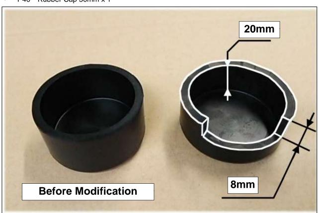
(23) Install the Rubber Cap 50mm modified in 2.(24) to the position of the air cleaner where the resonator was removed in 2.(20).
