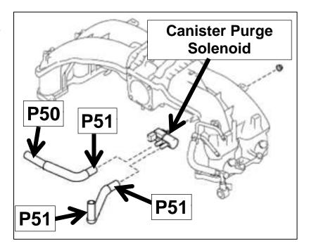
(30) Reinstall the canister purge solenoid. Place the throttle body and A/C compressor back in place.
