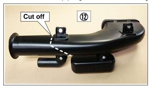
(25) Cut the blow-by hose at 15mm from the end as shown in the diagram below.
