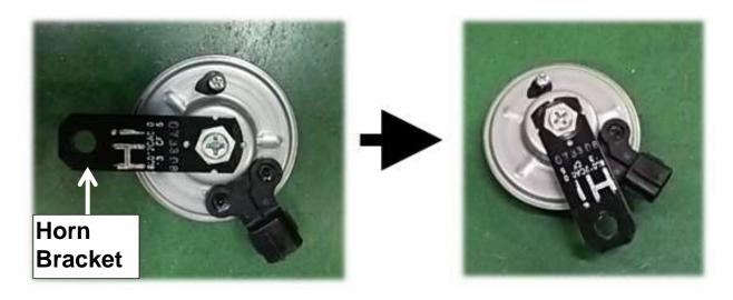
(8) Remove the plastic guide and clip from the horn and outside temperature sensor.
