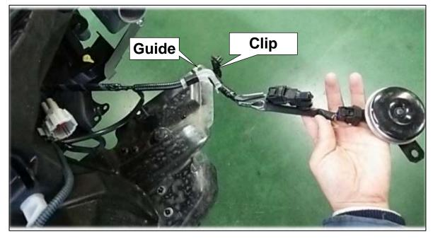
(9) Install the outside temperature sensor and horn to the A/C condenser bracket install in 2.(2).
