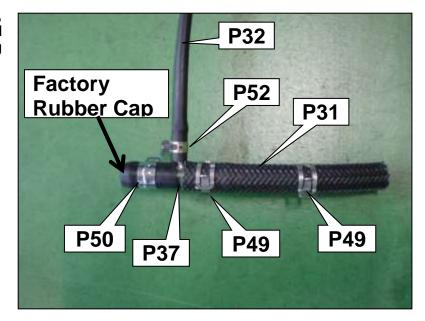
(11) Install the Hose 10mm to the intake manifold.
