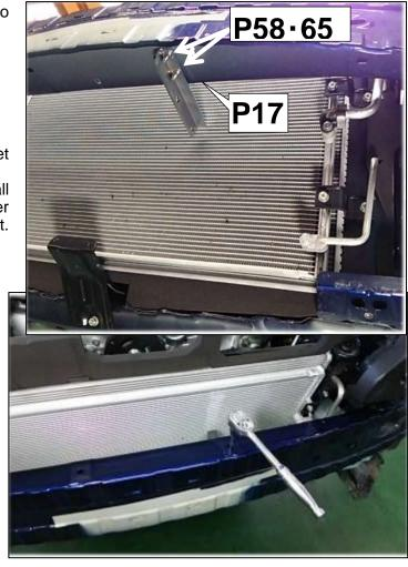
(5) Shave 2mm of the pipe clamp on the A/C condenser of the passenger's side as shown below.
