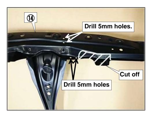
(14) Cut off the portion of the idler pulley installing part of ③alternator bracket removed in 1.(24) along the dotted line shown in the diagram on the right.
