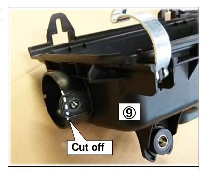
(22) Cut the Rubber Cap 50mm as shown in the diagram below.
