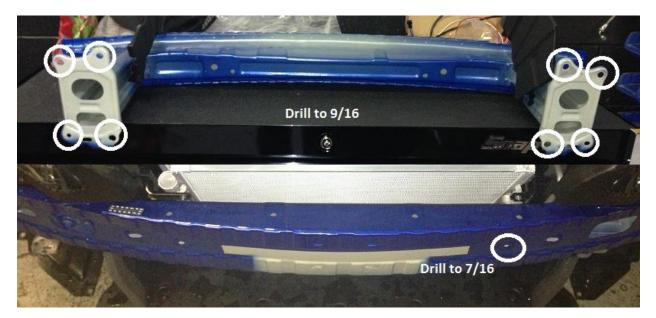
Mount the intercooler with the tabs behind the bumper support. Mount it with the supplied 7/16 bolt, nut and lock washer. Reinstall the first plastic front under panel.
