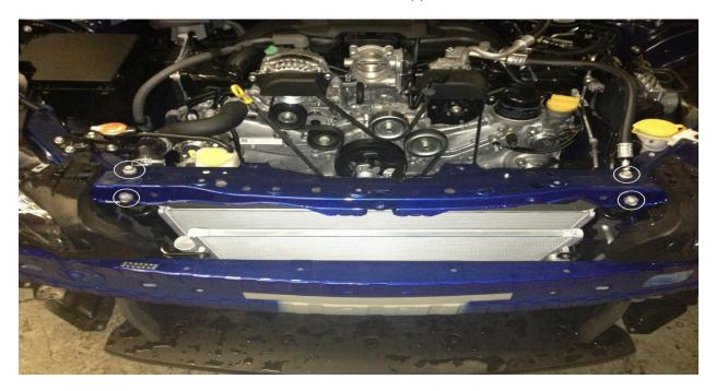
Remove the washer fluid reservoir.
