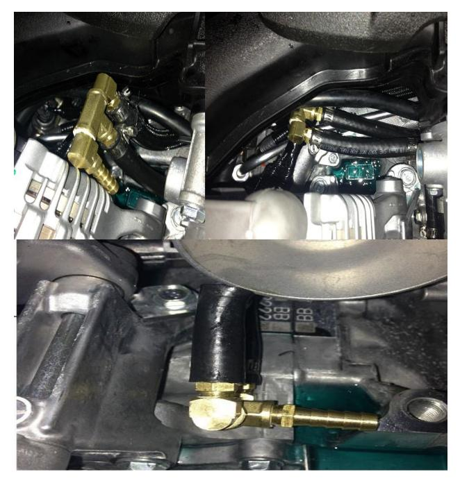
The easiest way to install the fitting is to install the banjo onto the water line first and then bolt it to the turbo with a 21mm wrench. The front water line will come with a heat resistant sleeve.
