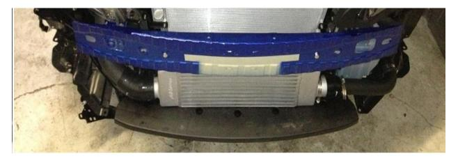
Remove the plastic pieces on the support bar. They are on with (1) push pop rivet on each side. Drill two plastic tabs on each piece to remove the front portion. Reinstall on the car. Reinstall the plastic pop rivet on the bottom of each plastic piece to the front under panel.
