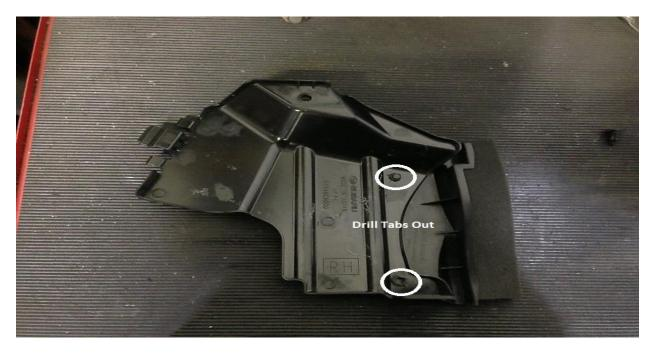
Trim some of the plastic with a utility knife to make room for the intercooler piping. You will also need to trim part of the washer resivoir tab.
