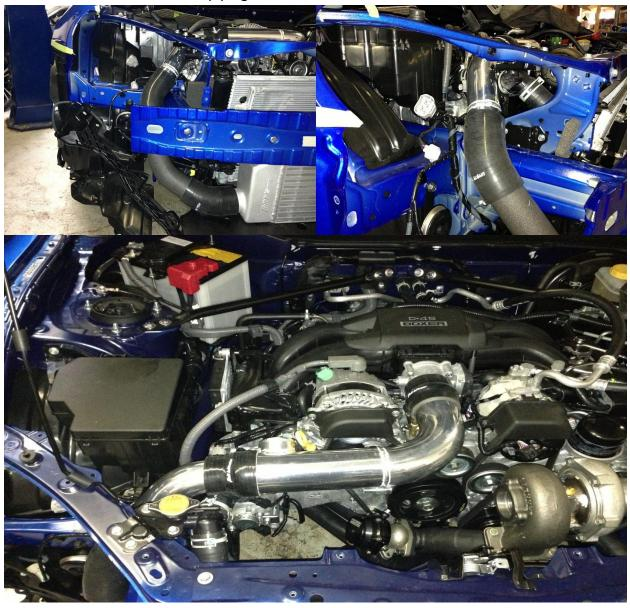
Install the cold side intercooler piping and BOV. Install the MAF sensor.
