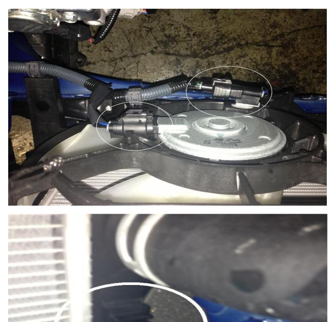
Pinch clip and slide forward to remove the stock fan.
