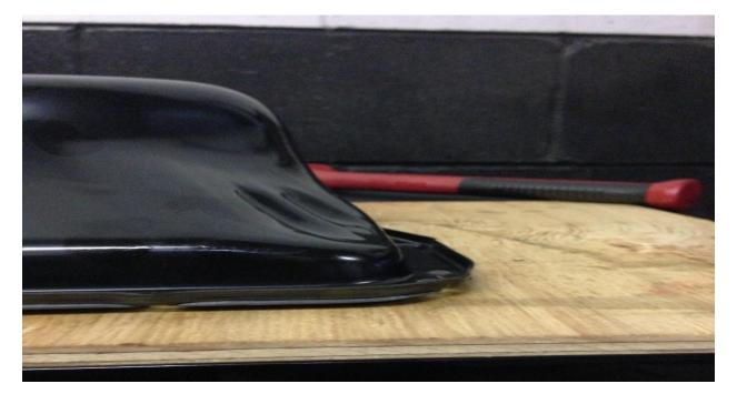
Using a razor blade, scrap off the old RTV from the oil pan. Wipe down the and clean the surface of the engine.
