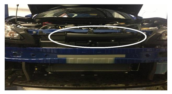
Remove the (6) 12mm bolt holding the bumper support in place. There are four bolts up to and two on the bottom. Disconnect the latch and set the support bar aside.
