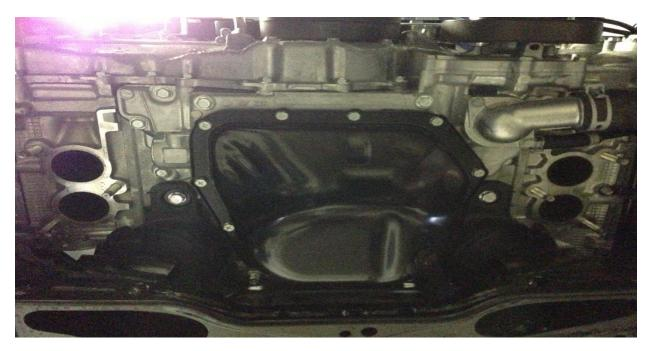
The oil pan will have a slight bend on the corner of the pan. Remove the two round gaskets and turn the oil pan upside down and using a soft rubber hammer tap the corner to flatten it back out. It helps to lay it face down on a piece of wood.
