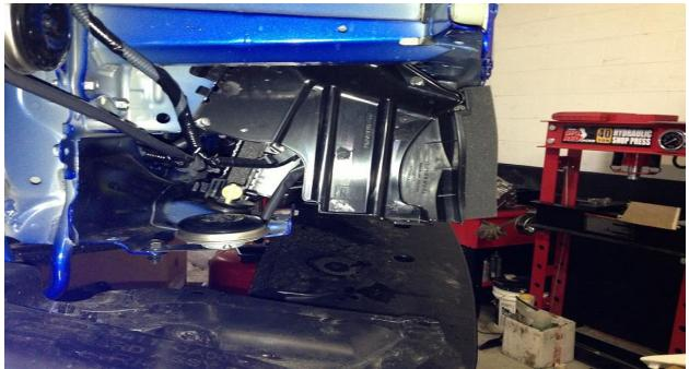
Remove the (8) 12mm bolt holding the bumper support and the two plastic pop rivet. Set the bumper support aside. There is some modification to fit the intercooler in place. Remove the (4) 10mm bolts holding the A/C condenser in place.
