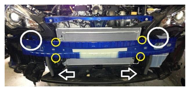
Install the slim fans. Slip the tie through the fan mount with the cushion between the fan and the radiator. Stop when you see the tie at the other end of the radiator and attach the clip to the end. The easiest way to do this is to pass the tie all the way through the A/C condenser and the cut off the excess part of the tie.
