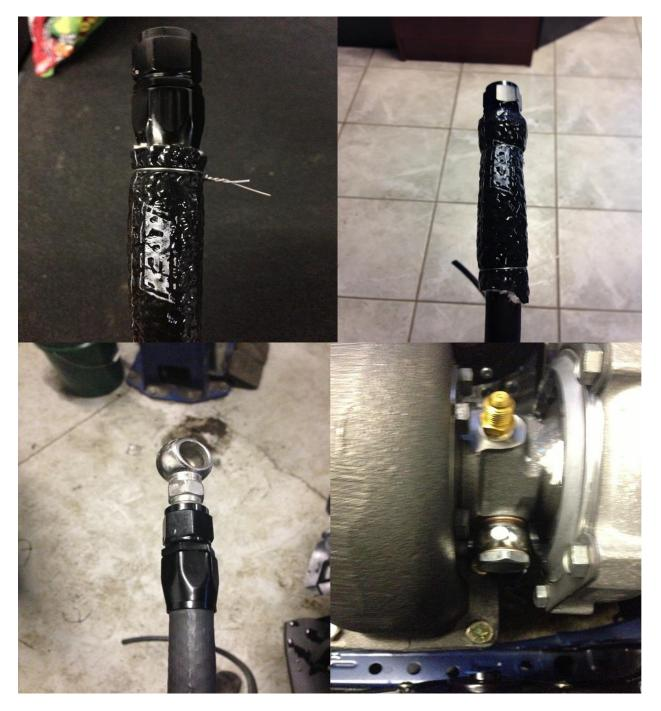
Remove the small bracket on the driver side frame rail. Route the water lines to the right of the oil fill and underneath the A/C compressor to the brass fitting.
