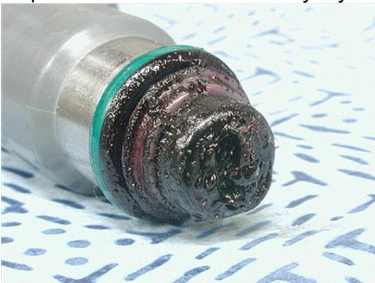
Deposit after 60 000 km in High Speed-test
