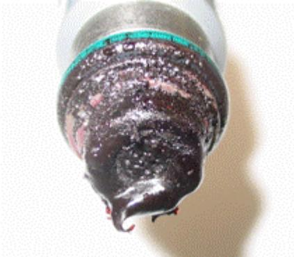
Injector deposit after one tank of clean up
