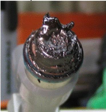
Injector deposit after 100 km on gasoline
