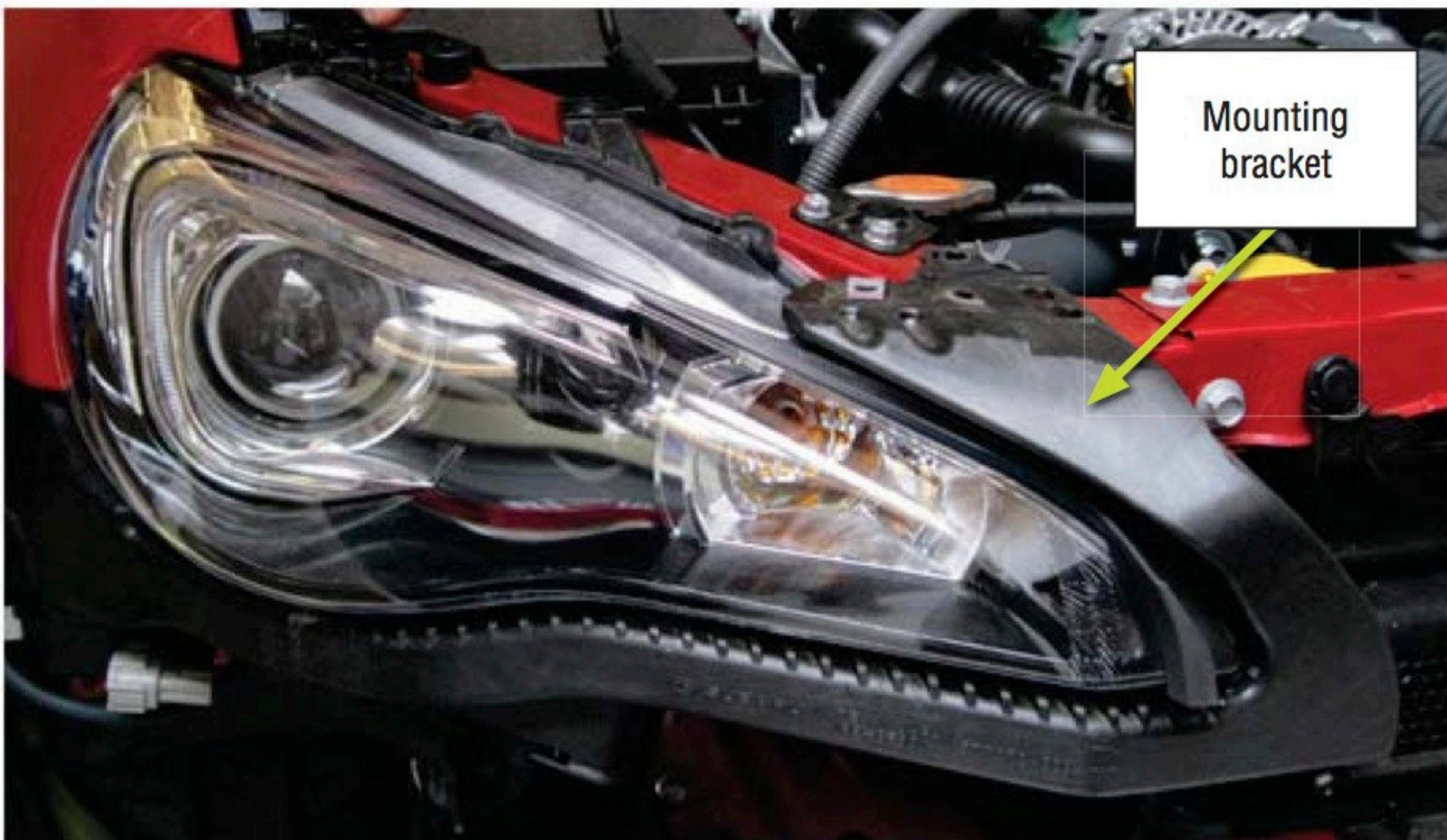
The design of the bracket has been revised to provide increased retention capabilities for the bumper fascia. Shown below is a comparison between the original-style bracket and the new-style.
