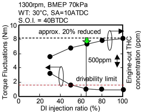
Fig. 19 Effect of simultaneous injection at fast idling
