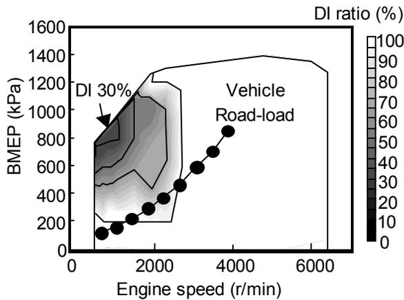
Fig.16 Final injection strategy of DI injection ratio
