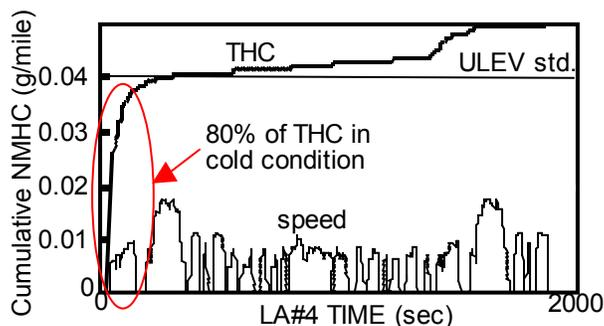
Fig. 17 Transition of HC emissions for FTP mode
