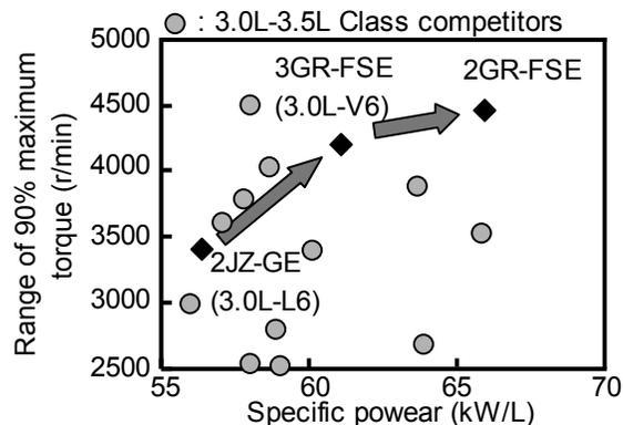
Fig.23 Full-load performance characteristic of the 2GR-FSE
